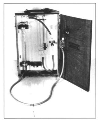
Figure 6. A Haldane gas analysis apparatus for measuring  $CO_2$  in a gas sample. The sample is drawn into the bulb of the water-jacketed pipette on the left, and the  $CO_2$  is absorbed by potash when the gas is driven over into the tubing on the right by raising the mercury, seen here hanging from a rack and pinion on the door of the apparatus.
